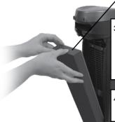
3. Take the new filter out of the plastic bag; distinguish the front side from the back side of the filter. The front side has the black foam layer, known as the pre-filter, which should be facing out when inside the unit, insert into the air cleaner with the arrow pointing inward.
