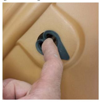
2. Press the seal back into a round – the tab should be flat against the barrel
