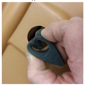
1. Crimp the threaded seal into a "U" then insert into the hole from the outside of the barrel
