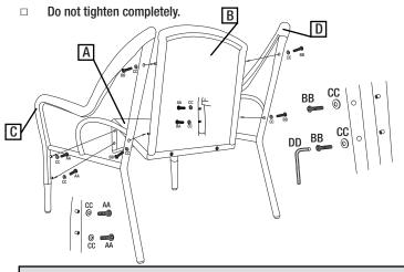
Note: For easier alignment and assembly, attach the lower panhead Allen bolts (AA) before the upper panhead Allen bolts (BB).
