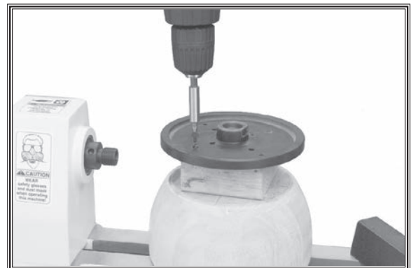
Figure 35. Example of mounting workpiece to a faceplate using a backing block.
