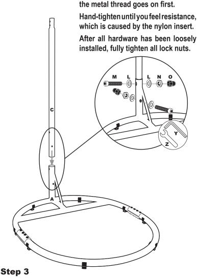
Slide Straight Pole (C) into Base Back (A) and align the holes. Secure the pole using Bolt (M), Washer (L), and Lock Nut (N). Tighten the hardware using Large Hex Key (Y) and Spanner (Z). Place Large Hex Nut Cap (O) over the lock nut.
