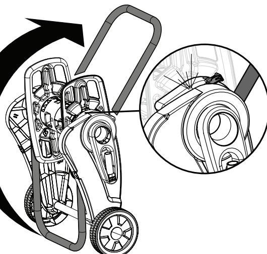
Swing the folding handle up into position until it snaps in place.
