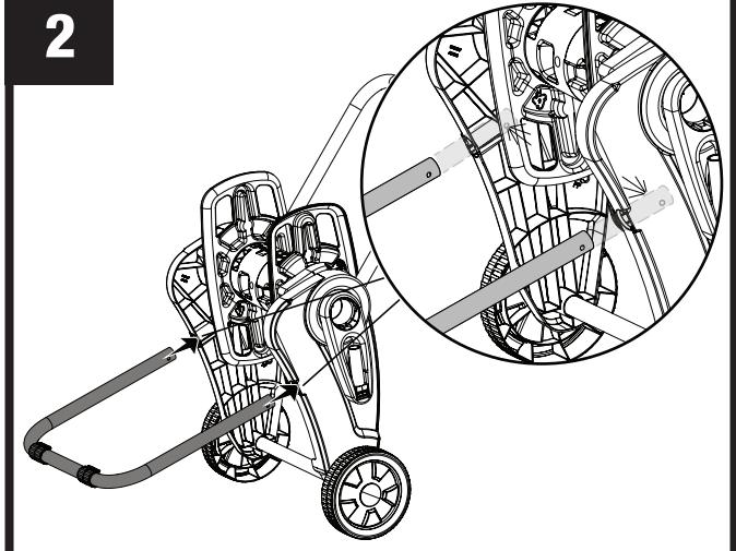
Insert the leg tube into the side frames until it snaps in place on each side
