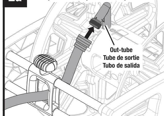
**Reel With Hose Guide** – Insert garden hose through hose guide and connect to out-tube. Turn on water supply and check for leaks. If necessary, re-tighten connections.
