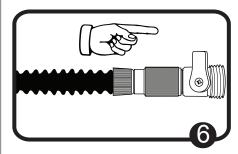
6. Once the HOSE is fully expanded, turn the ON/OFF valve on. Now you can use the hose freely.
