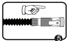
5. Turn on the water source, increase its pressure gradually while the hose manually expands three times its original length.
