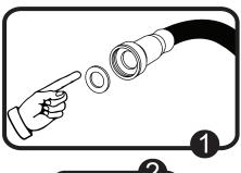
1. Place the rubber washer firmly inside the female coupling to prevent water leakage before using the HOSE. At first usage, fill the Hose to expand it, then Gently stretch it free from its tightness in its outer bent covering material. After which, pour out the water from the Hose and use the hose normally.
