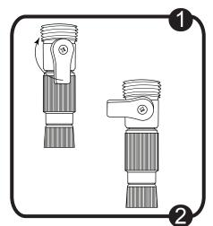
1. Firstly, turn the ON/OFF valve at the HOSE end OFF.
