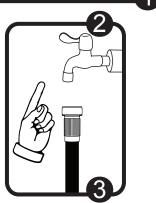
2. Into the source spigot, attach/connect the female end of the HOSE.
