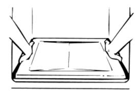
The oven bottom has a porcelain enamel finish. To make cleaning easier, protect the oven bottom from excessive spillovers. This is particularly important when baking a fruit pie or other foods with high acid content. Hot fruit fillings or foods that are acidic in content, such as milk, tomato or sauerkraut, and sauces with vinegar or lemon juice, may cause pitting and damage to the porcelain enamel surface.
