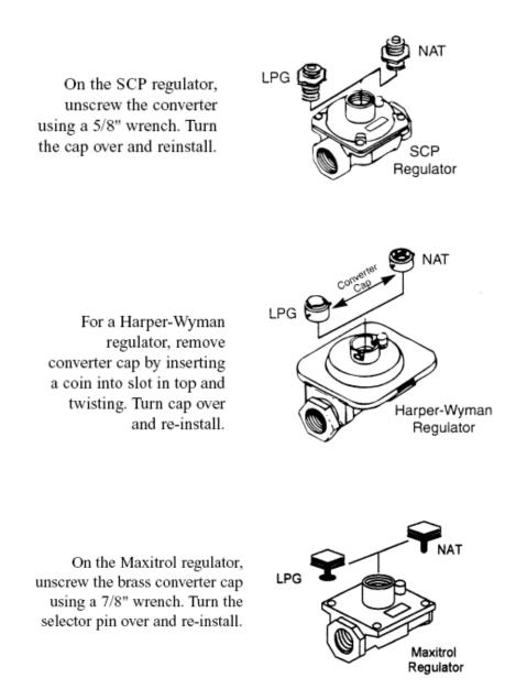
**Note:** What you read on the converter cap or plunger is the type of gas for which the regulator is set. If yours reads NAT, the regulator is set for natural gas. If yours reads LP, the regulator is set for LP.
