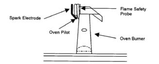
Ovens with Standby Pilot Battery Spark Ignition
