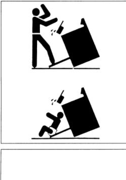
To reduce the risk of tipping the appliance by abnormal usage or improper door loading, the appliance must be secured by properly installing the anti-tip device packed with the appliance. To check if the device is installed and engaged properly, carefully tip the range forward. The Anti-Tip device should engage and prevent the range from tipping over.
