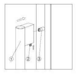
Locate the handle(1)over the pins(3)of the door and tighten the handle by screwing the Allen key grub screws(2)
