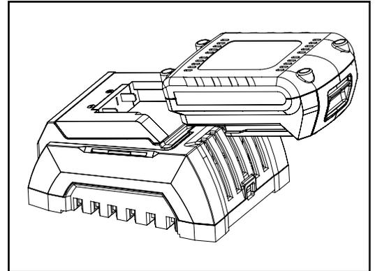
**NOTE:** Batteries may become warm while charging. This is normal. If the battery is hot after continuous use in the tool, allow it to cool down to room temperature before charging. This will extend the life of your batteries.
