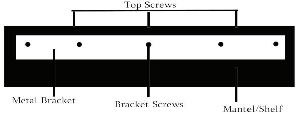
Step 1. Remove all screws from the bracket. Both bracket screws and the top screws.
