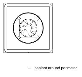
4. Place RBSF above opening by sliding flange in place underneath shingle. Using a #8 or #10 screw(or nails) should be placed approximately a distance of 4 inch on center on all 4 sides.
