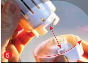
5 Attach Ceramic filter (included) to the Tank Cap by aligning the lock tabs on both and turning the cap counterclockwise to lock. When attached properly the Filter will not fall from the Tank Cap.
