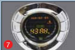
**LOW Water** – When the Tank is out of water the “waterless” indicator will appear in the display, you will hear 3 beeps and the automatic safety shut-off will turn the Ultrasonic Nebulizer & unit OFF.
