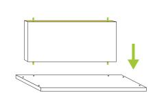
Carefully remove the protective layer on the Back and Vertical zBoards, making sure not to remove the 3M adhesive.
