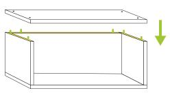
Align Top zBoard and press firmly to secure unit together.
