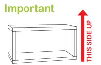
**CAUTION** placing unit on its side or back will compromise structural integrity. Use right side up.
