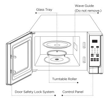
NOTE: Do not remove the mica plate covering the wave guide in the oven cavity.
