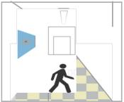
When motion detected, insufficient daylight.Light ON.
