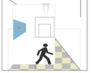
After last detection, the light will be dimmed down to the stand-by dimming level(10%,30%,50%).
