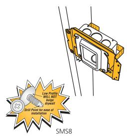
The CADDY MEB1 extends stud depths to 4". The bracket has built-in support legs to reduce box movement when used with EMT. It is ideal for flexible conduit, ENT, MC, AC or nonmetallic sheathed cable.
