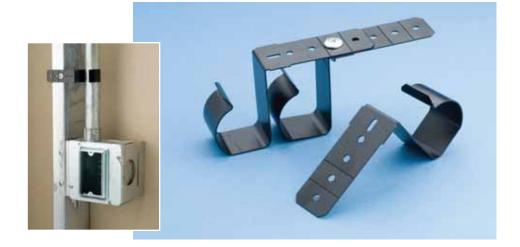
CADDY<sup>®</sup> Screw-On Conduit Supports from ERICO<sup>®</sup> securely attach EMT conduit or MC/AC cable to wood and metal studs. The supports comply with NEC<sup>®</sup> 358.30(A) and CEC<sup>®</sup> rule 12-1404 which requires conduit support within 36" of an electrical box and also comply with CEC Rule 12-618 which requires support of an armored cable within 12" of an electrical box.
