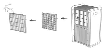
**WARNING**: It is strongly advised to rinse the filter every two weeks. Any dust blocking the filter will potentially affect the machine's functionality.
