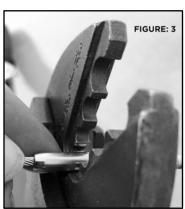
4. Bring the handles of the crimping tool together until the crimping head is closed
