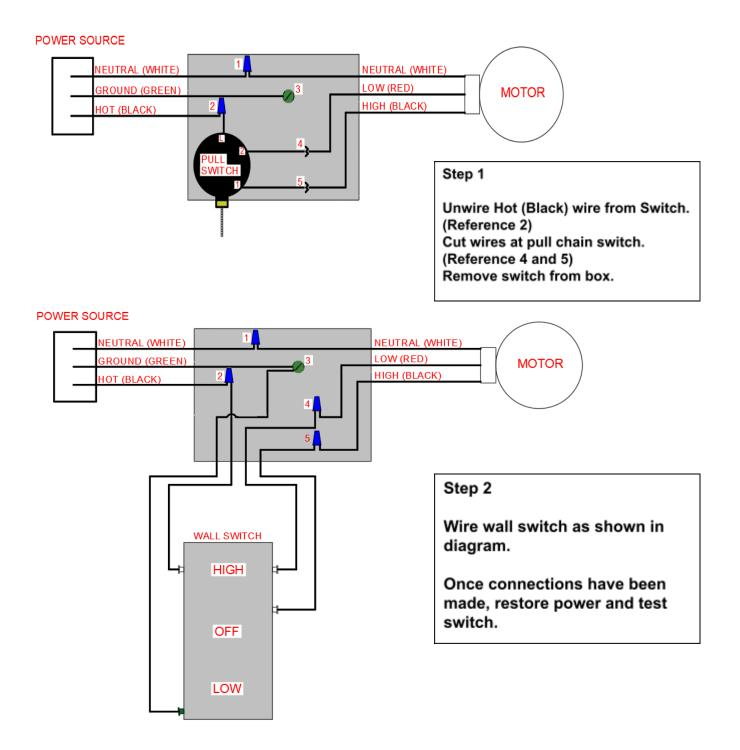
NOTE: Follow all Electrical Codes when installing. Remove power from the circuit before performing electrical work.
