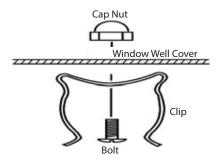
Snap window well cover onto rim of window well.
