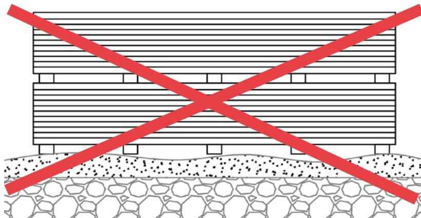
NewTechWood products shown above on an uneven surface which will make the products prone to warping and distortion.
