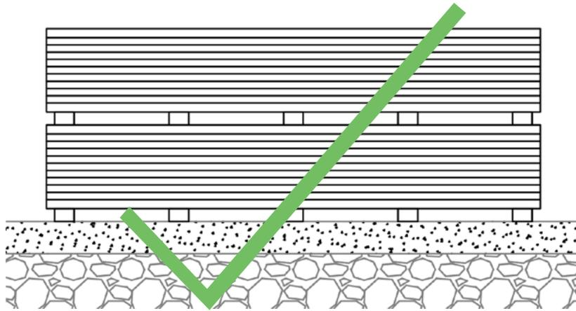
NewTechWood products shown above put on a flat surface on joists, this is the correct way for storage.
