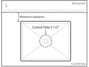
2. Once the placement has been determined. Mark the center of the drain hole and set aside the vessel sink. Draw a 3 1/2 inch diameter circle around the center of the drain hole. Use a jigsaw or a power tool to cut the opening on the mounting surface.
