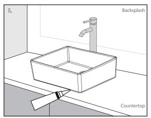
5. Install the sink and connect P-trap to the drain and check for alignment. Apply some caulking around the base of the sink to seal any gap between the sink and the countertop. (\*NOTE: After the installation is completed. Turn on the faucet and let it run for few minutes and check for leaks around the sink above and under the countertop.)
