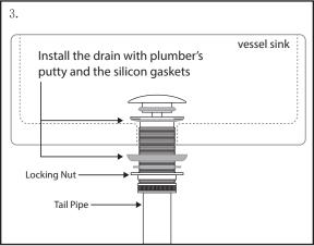
3. Attach the pop up drain to the ceramic sink as shown. It is recommended to use plumber's putty with the silicon gaskets to prevent any possible water leak. Make sure the drain is properly secured to the vessel sink.
