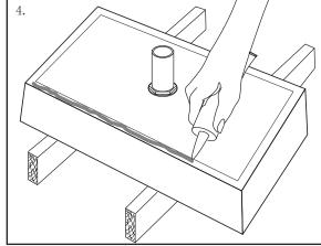
4. Place the assembled vessel sink through the 3 1/2" opening on the counter top and check for level and fit. Plumber's putty can be used to level the sink. Apply silicon adhesive around the bottom rim of the sink as shown.
