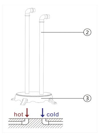
3 Lock the body(#4) to the elbow of supply columns(#2).
