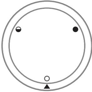
For a Normal Soak; position the handle so that the arrow is as shown below.
