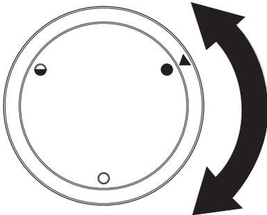
To close the Overflow position the handle so that the arrow is as shown below.
