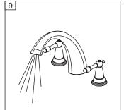
Important: After installation is completed, Turn on water supply and allow both hot and cold water to
