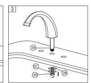
Insert spout shank (3A) through the center hole of the tub. Then from underneath, place rubber washer (3B) and metal washer (3C) onto the bottom of the spout body (3A) and tighten with mounting nut (3D).
