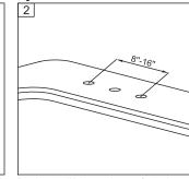
Drill three 1-1/2" diameter holes in finished surface. Note: Space holes according to the
