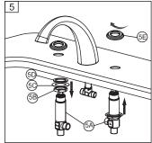
Place mounting nut (5B), metal washer (5C) and rubber washer (5D) onto valve body (5A). From underneath the tub, insert valve body (5A) though holes on the right (cold) side. From above, thread flange (5E) onto valve stem (5A). Tighten mounting nut (5B), so that the flange sits flush to the surface of working area. Then insert the other valve body thought hole on the left (hot) side and install in the same way.
