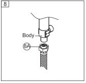
Connect water supply lines (8A). Use supply lines with 1/2" IPS faucet connections.
