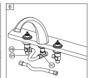
Connect the flexible water supply hose (6A) to the bottom of the valve bodies (6B) as shown Align T-tube (6C) in a position which will allow maximum clearance to connect hoses. Carefully bend the hoses to fit the available space. Carefully thread the hose couplings to the sides of the T-tube.
