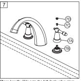
Place handle (7A) onto the left (hot) valve stem (7B). Place screw (7C) through the socket on top of the handle and thread until handle is securely tight. Attach decorative (7D) button onto the lever socket. Place the other handle assembly onto the right (cold) valve stem and install the same way.
