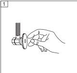
Shut off water supply. Remove old faucet. Clean sink surface in preparation for new faucet.
