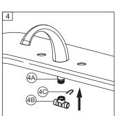
Push the T-tube (4B) onto the end of the spout tube (4A) until it seats. Insert ring (4C) through the groove on the spout tube end. Make sure the T-tube is aligned at an angle which will allow maximum clearance to connect hose.
