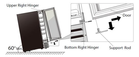
3. Unscrew the upper hinge and bottom hinge.
