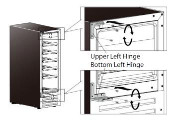
6. Rotate the door 180° so that the top is now the bottom, and install it by attaching the support rod with screws.
