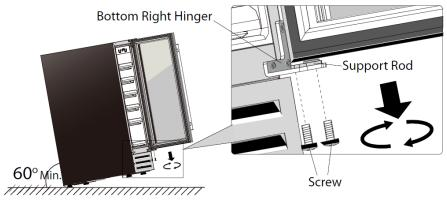
2. Remove the door from the upper hinge and take out the support rod.
