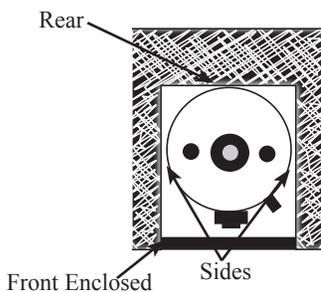
**▲ WARNING: Combustible construction refers to adjacent walls and ceilings and should not be confused with combustible or flammable products and materials. Combustible and/or flammable products and materials should never be stored in the vicinity of this or any gas appliance.**
