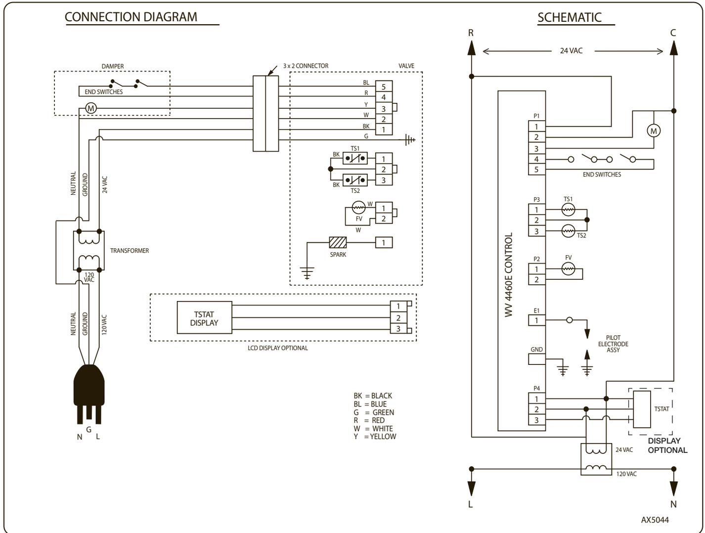
**⚠ CAUTION!** Label all wires prior to disconnection when servicing controls. Wiring errors can cause improper and dangerous operation. **VERIFY PROPER OPERATION AFTER SERVICING!**
