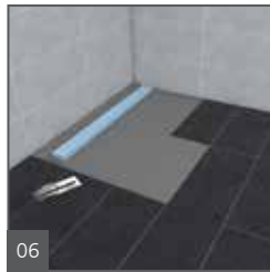
06 Use the foam block (provided) as a spacer for thinset mortar.
