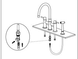
Rotate the gasket and nut to lock
