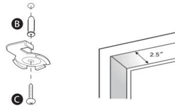
**Step 4** Attach the track to the mounting brackets. We recommend additional hand to finish this step.
