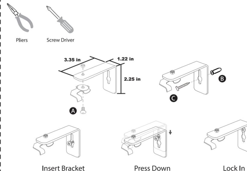
**Step 4** Attach the track to the mounting brackets.
