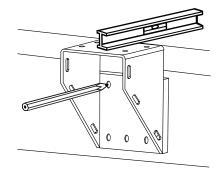
**5.** Remove the bracket and drill 3/16" pilot holes at the marked positions.
