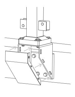
**9.** Attach remaining brackets to deck structure following steps 3-6 above.
