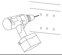
6. Place the bracket back into position and attach the bracket to the fascia board using the 6 - 3/8" x 3" lag bolts supplied. Ensure that the top of the bracket is level and plumb (shim as necessary).
