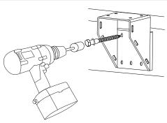
**7.** Attach the post to the fascia mount bracket using the 4 - 1/4" x 1 1/2" machine bolts, washers and locking nuts supplied. Ensure post is plumb (shim as necessary).
