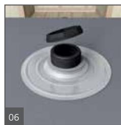
06 Tighten the gaskets firmly to the bases' steel ring using the locking nut. Make sure the drain body is still safely received in the valve-bead of sealant. Smooth out excess sealant over the drain body's flange surface.
