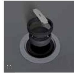
60 minutes after initial installation of the drain with wedi Joint Sealant tighten (squeeze) the rubber caulking gasket firmly with the caulking nut (use a flat headed screwdriver) and finally insert the plastic frame and strainer on top (without adhesive). The frame and strainer will be held in a grout joint only once tiling commences. Do not tighten the gasket prior to 60 minutes after the threaded drain part was sealed into the shower base.
