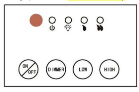
button will turn it off. Similarly, a <HIGH> button press will switch the heater to high-power status when **w** is dark, and turn it off when **w** is brighten up.
