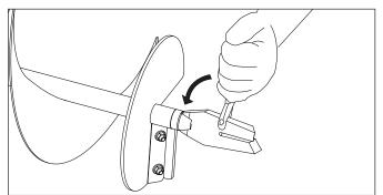
Then, using your hand, unscrew the fishtail bit completely. Replace with new part.
