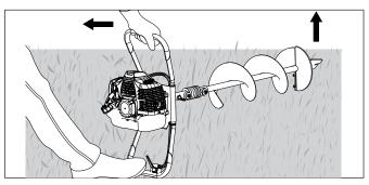
6. Holding the unit firmly, pull the recoil starter grip 2 times to prime with fuel, then pull until engine starts. Use short pulls and do not allow the rope to snap back. Do not pull more than 6 times.
