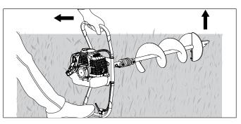
5. Holding the unit firmly, pull starter handle until engine starts. Use short pulls and do not allow the rope to snap back.
