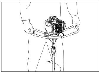
8. After the engine runs for 10-15 seconds, move the choke lever to the run position.
