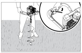
**CAUTION:** The auger bit will continue to rotate for a few seconds after the throttle/speed control is released.
