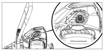
2. Use a spark plug socket tool, or a 3/4 in. (19 mm) socket to remove the plug.
