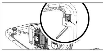
3. Set the choke lever to the CHOKE position.
