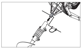
2. Carry the power head by the handle that does not have the throttle/speed control with the recoil starter against your leg so the fuel tank cap is pointed skyward while carrying the auger bit in the other hand, held by the shaft.
