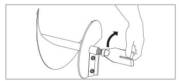
To tighten securely, grasp the auger bit shaft with one hand while placing an adjustable wrench on the fishtail bit point and tighten until it is securely in place.
