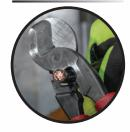
• Cut 4/0 aluminum, 2/0 soft copper, 100-pair 24 AWG communications cable
