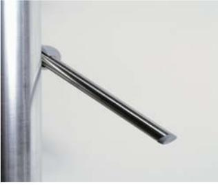
Stainless Steel Tubes (PA5) are installed through the fittings provided on your posts. Loosen set screw on each fitting to slide your tubes through, then tighten each set screw securely. For seamless tube to tube connections, splice them at the post fittings. Use the plastic caps provided to finish tube ends. It is recommended that an angle grinder be used to cut tubes.
