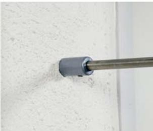
Wall terminals for tube filling (PA11) connect your steel tubes individually to a perpendicular wall. Line up your tubes against the wall to mark connection points. Use the screws provided to secure fittings to wall. While securing handrail connector with backing material in place is strongly recommended, if adequate backing material is not in place, a toggle bolt or heavy duty drywall anchor can be used. (Sold separately). Then slide tubes into fittings and tighten set screws securely.
