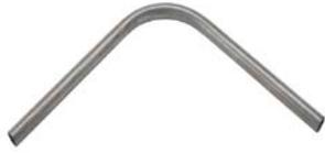
90° corner for tube or cable (PA25) can be installed from post to post in the fittings provided, to finish corners. Loosen set screws on fittings and install in the same manner as steel tubes. Tighten set screws securely. When using cable, after installing, thread cable through corners, and continue cable to next post.
