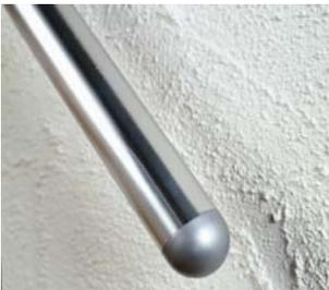
Handrail endcaps (PA7) are installed to finish your run of wood or aluminum handrails. Using an allen wrench (not supplied), remove the plug from the end cap. Drill pilot hole (in wood handrails) or use existing hole (in aluminum handrail), and mount plug onto handrail with screw provided. Then replace the cap, and tighten set screw securely. For wood handrails, it is recommended that you use a drilling template (PA21, sold separately) to drill 1/8" pilot holes on center.
