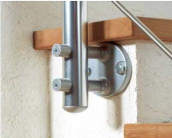
Side Mount Posts (PA2) can be used with any of the PROVA in fills. (Acrylic glass, stainless steel cable, or stainless steel tubes.) Always use all of the provided mounting screw holes. Never cut or drill new holes in your post base. For uneven surfaces, use the post leveler (PA14, sold separately). For stair treads that extend, use the spacers (1 7/8" PA12 or 2 7/8" PA13, sold separately). Set posts no more than 4' on center.
