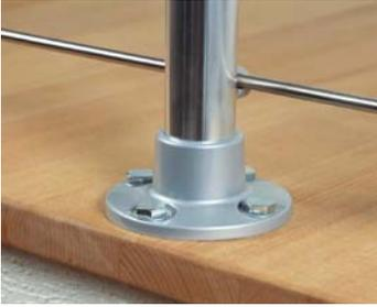
Top Mount Posts (PA1) can be used with any of the PROVA in fills. (Acrylic glass, stainless steel cable, or stainless steel tubes.) Always use all of the provided mounting screw holes. Never cut or drill new holes in your post base. For uneven surfaces, use the post leveler (PA14, sold separately). Set posts no more than 4' on center.
