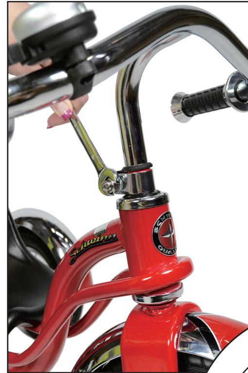
Note: Ensure minimum insertion mark (pictured) is not visible.
