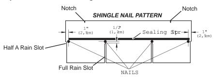
! NEVER DRIVE FASTENERS INTO OR ABOVE SEALING STRIPS.
