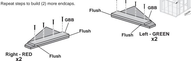
Locate endcaps flush with upper trim and corner trim. Secure each endcap from inside of shed with (4) 1-1/4" screws, as shown (Fig. A).
