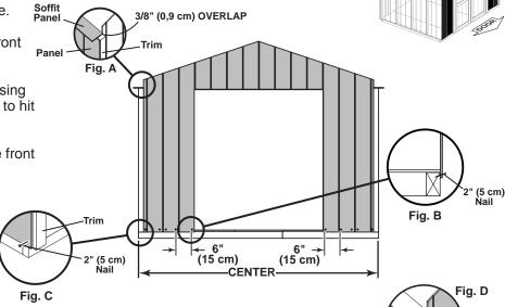
Be sure the measurement between the panel edge and the trim is the same along the entire length. Then secure with (1) 2" nail in the upper corner (Fig. D).
