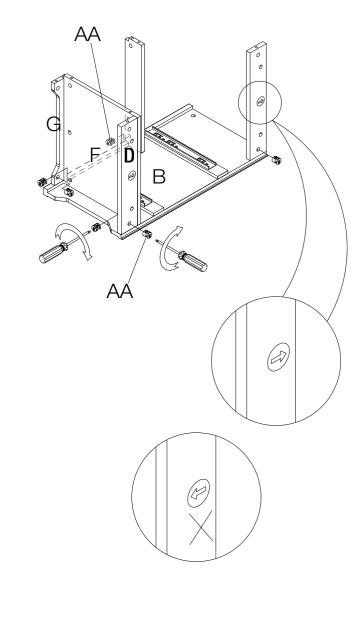
Big cam lock Big cam lock bolt Wood dowel
