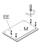
d) Insert wood dowel(CC) into panel(J&K), then rotate the cam lock(DD) tight to assemble panel(J&K) and panel(M).
