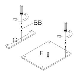
□ b) Assemble the panel(G) and panel(D) with panel(F)
