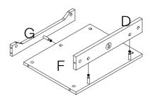
□ c) Insert and rotate cam lock(AA) to assemble panel(G),panel(D) and panel(F)
