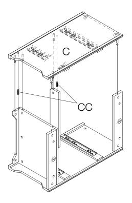
$\hfill\Box$  c) Assemble panel(C) by inserting and rotating the cam lock(AA).
