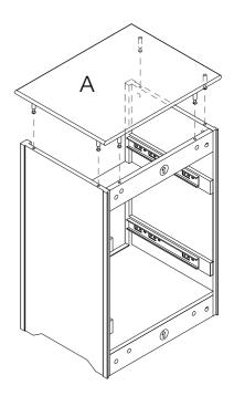
□ c) Insert and rotate cam lock(AA) to assemble panel(A).
