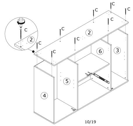
Attach No.2 plate to No.3, No,6, No.5 and No.4 plate, and fix with screw(C) as shown.
