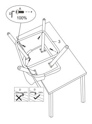
WARNING!! Over tightening could lead to issue during leveling assembly step and product wobble. Tighten only until secure and stable.
