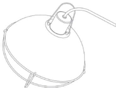
WITH HANGER INSTALLED INSTALADA CON COLGADOR
