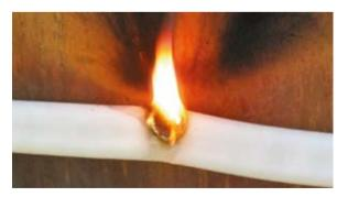
The heating of surrounding materials creates a carbon remnant that acts as a high impedance conductor. As the carbon path extends, the by-products of the arc increase the available fuel source, magnifying the likelihood of a fire.
