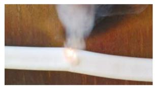
Arcing faults, which can and generally do go undetected by traditional circuit protection means, can reach extraordinarily high temperatures — upwards of 9,000 degrees Fahrenheit.
