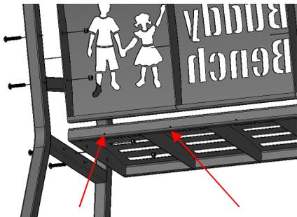
Note the water drain hole location on each seat section. For the Seat section, the holes should be facing the back of the bench when fastened to the bench ends.
