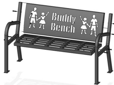
Using the supplied hardware (Items 4 & 5) and the supplied Phillips driver bit (Item 6), loosely assemble the Seat section (Item 1) to the (2x) Bench End Frames (Item 3). **Note:** This may be easier with two people.
