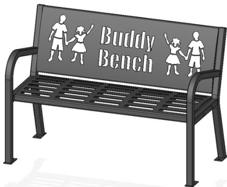
Verify all hardware is tightened (do not over tighten). Place the bench where you would like to permanently install, and mark the solid surface below the bench through the holes in the four feet. Using concrete anchors on a solid surface, drill a 3/8" diameter pilot hole 1-3/4" deep into the solid surface, and secure the bench to the ground using the supplied 3/8" hardware.
