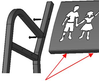
Note the water drain hole location on each seat section. For the backrest, the holes should be facing the ground when fastened to the bench ends.
