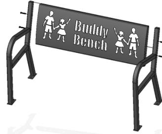
Using the supplied hardware (Items 4 & 5) and the supplied Phillips driver bit (Item 6), loosely assemble the back rest (Item 2) to the (2x) Bench End Frames (Item 3). **Note:** This may be easier with two people.
