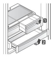
To install, slightly tilt up the front, insert the drawer into the frame and push it back into place.
