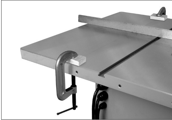
Figure 6-5: leveling extension wings, method 2
