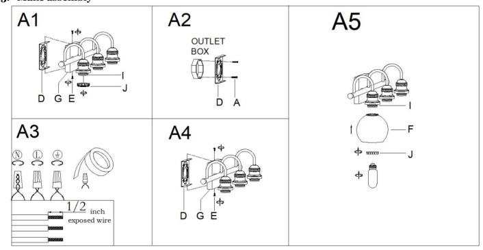
Step A1: Unscrew the studs(E) from the back plate(G) then gently remove the mounting plate (D). Unscrew socket ring (J) from socket (I).
