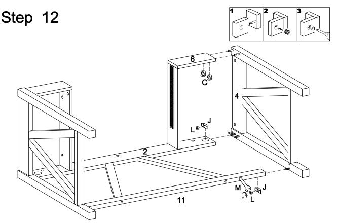
Insert side frame (4) into back panel (2) and parts (6,11), then insert and secure cam lock (C) to parts (6), and use wrench (M) to secure back panel (2) and parts (11) with half moon washer (J) and nut (L) to lock them.
