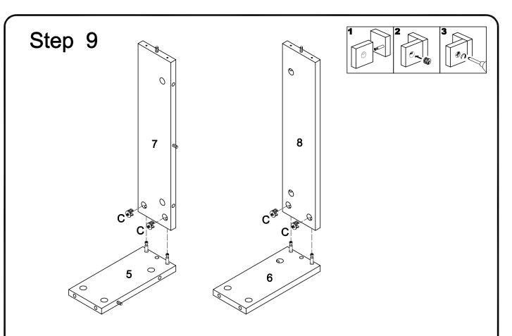
Insert parts (5,6) into side panel (7,8), then insert and secure cam lock (C) to side panel (7,8) to lock it.
