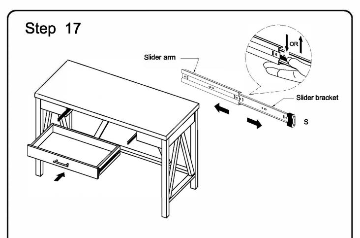
Press down/up the slider lock on slider bracket, then insert the drawer into slider arm to lock it.
