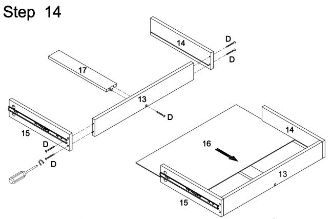
Insert parts (17) into drawer back panel (13) then secure it with screw (D). Secure drawer side panel (14,15) to drawer back panel (13) with screw (D). Slide drawer bottom panels (16) into grooves as per diagram.
