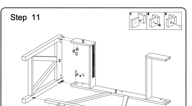
Insert side frame (3) into back panel (2) and parts (5,11), then insert and secure cam lock (C) to parts (5), and use wrench (M) to secure back panel (2) and part (11) with half moon washer (J) and nut (L) to lock them.
