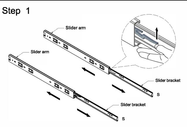
Disassemble drawer slider (S) by sliding the slider arm and slider bracket apart. Depress the small lever of the slider bracket and carefully pull the two pieces apart. Repeat this process for both drawer sliders (S).
