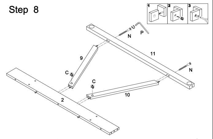
Insert parts (9,10) into back panel (2) and parts (11), then insert and secure cam lock (C) to parts (9,10), and use wrench (P) to secure parts (11) to parts (9,10) with bolt (N) to lock them.
