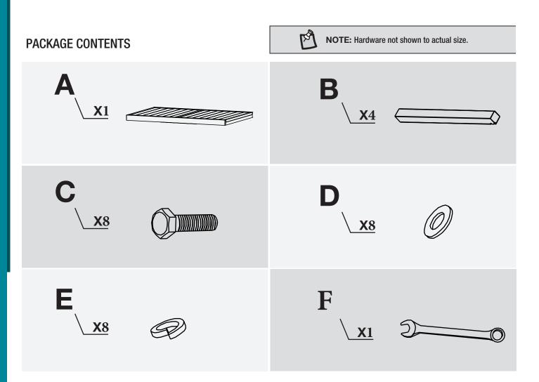
Once all connections are made, use F to tighten C, Dand E.
